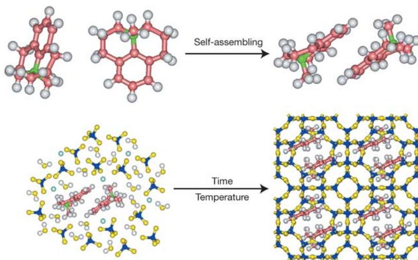
**Figure 1** Formation of the LTA structure from the supramolecular self-assembling of the OSDA molecules. See Supplementary Data. Atoms are colour-coded as follows: dark blue, silicon; light blue, fluorine; yellow, oxygen; red, carbon; green: nitrogen; grey, hydrogen.
