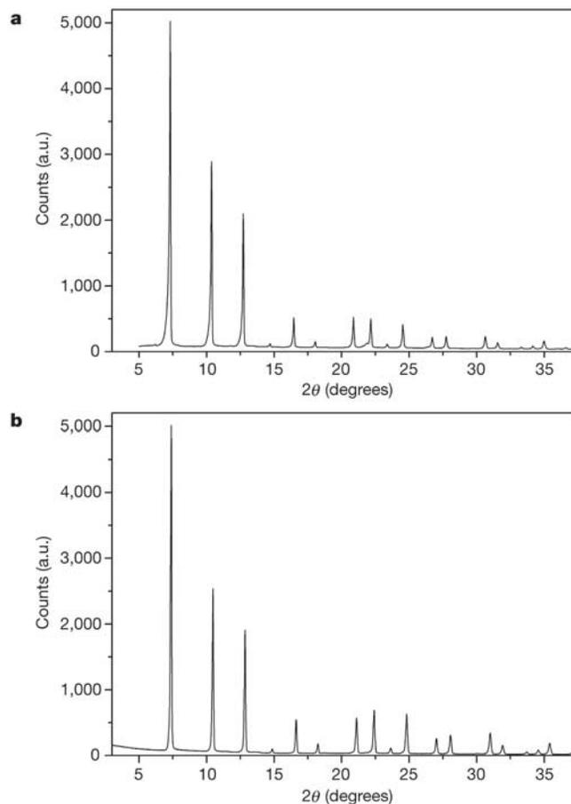
**Figure 2** X-ray diffraction patterns of calcined ITQ-29 materials. **a**, Ge-containing zeolite (Si/Ge = 2). **b**, Pure-silica zeolite.
